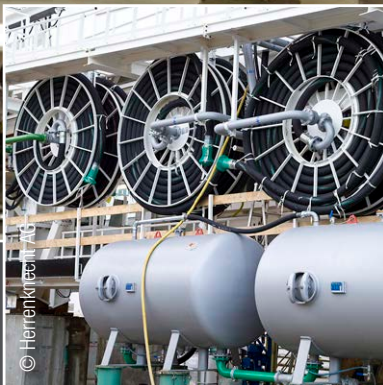
Hose reel during TBM build up for Herrenknecht "Bossler tunnel" - Germany
