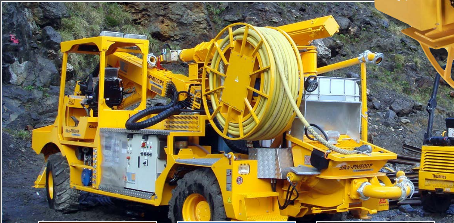
Hydraulic drive cable reel on shotcrete machine
