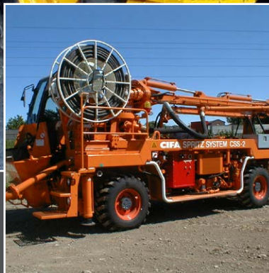
NAMI reel on shotcrete machine by Cifa
