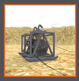
The "Dual Motorized Reel Unit" is a skid-mounted reeling machine that includes a level-wind reel for incoming power and an "umbilical cable" monospiral reel for the mobile machine. The magnetic coupler mechanism on the monospiral reel allows it to automatically pay out or take up cable as the machine moves. This creates a safer condition for the machine operator and protects the cable.
