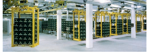
SingleFlexLine 0811 on an electrified monorail system in a brewery
