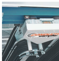
Motorized main cable trolley with magnetic switch for back reach limit stops
