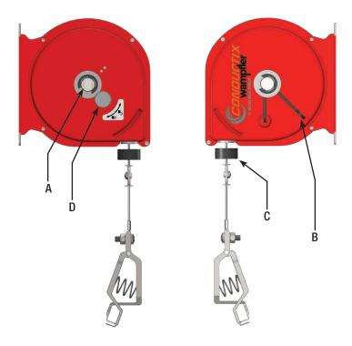
**INSTALLATION** - Mount the reel securely, Pull the grounding cable out to determine if the tension is sufficient for the intended use, If additional tension is needed, apply wrench to flats on the mainspring shaft (A), rotating counter-clockwise until the desired tension is reached.
